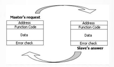
On the request telegram, the function code informs the addressed slave device about the action that must be performed. The data bytes contain the detailed information required for the function execution. For example, register address that must be accessed and the quantity of bytes that must be returned. At the end of the telegram, a cyclic redundancy guarantees the quality of the data transmission.
